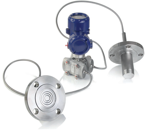
WIKA differential pressure transmitter mounted to two flange-type diaphragm seals via a capillary
